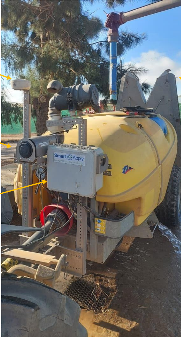
Control module – Send LIDAR data to solenoids for spray modulation
