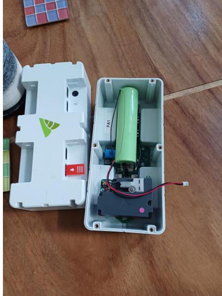
The Strella device on the inside with the different components that measure CO 2 , O 2 , RH, temperature and ethylene.
