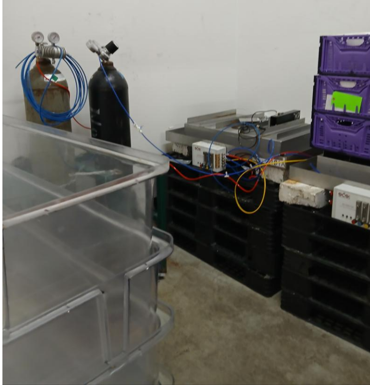
Example of experimental system to examine different gas combinations (concentrations of CO 2 and O 2 ) in storage trials.
