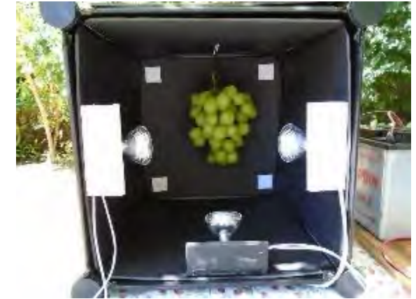
Figure 5. Example HSI and MSI collection process. SATI project “Physical and chemical bunch characterization of table grapes using machine vision”.
