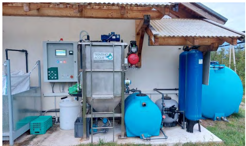
The bio-filter developed by Laimburg Research Centre to filter the irrigation water.
