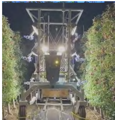
ADAM, a robot for precision management (harvest and spray) Robotic harvester from Advanced. Farm in the USA. They are the current leaders in the industry of robotic harvesting with a picking rate of 1500 apples per hour.
