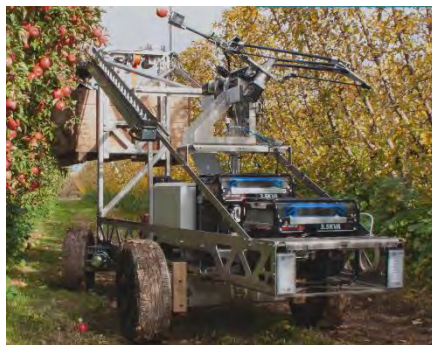
Robotic harvester from Ripe Robotics in Australia.
