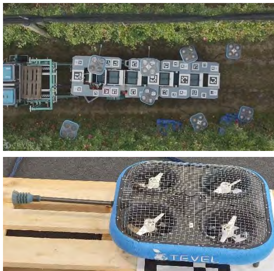
Harvesting drones from Tevel in Israel. Although it still has challenges, this flying robotic harvester showed the most promise in terms of height of operation, accessibility in orchards, dual sided harvesting etc.
